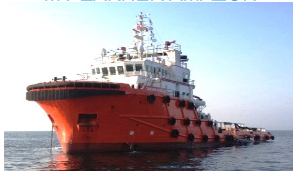
58.70 M ANCHOR HANDLING TUG SUPPLY VESSEL DP1 FIFI 1
